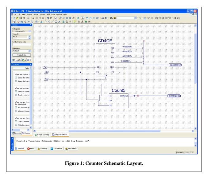
differently ordered than in Fig. 1. Test your design by creating a Testbench Waveform and running the simulation program to see the response of the counter. Be sure to make the clock stream long enough, so that more than 60 output counts are observed. This will ensure that the full functionality of the counter is tested. If your design is successful, create a schematic symbol for your new counter and verify that it is available as a symbol on the schematic entry page.
