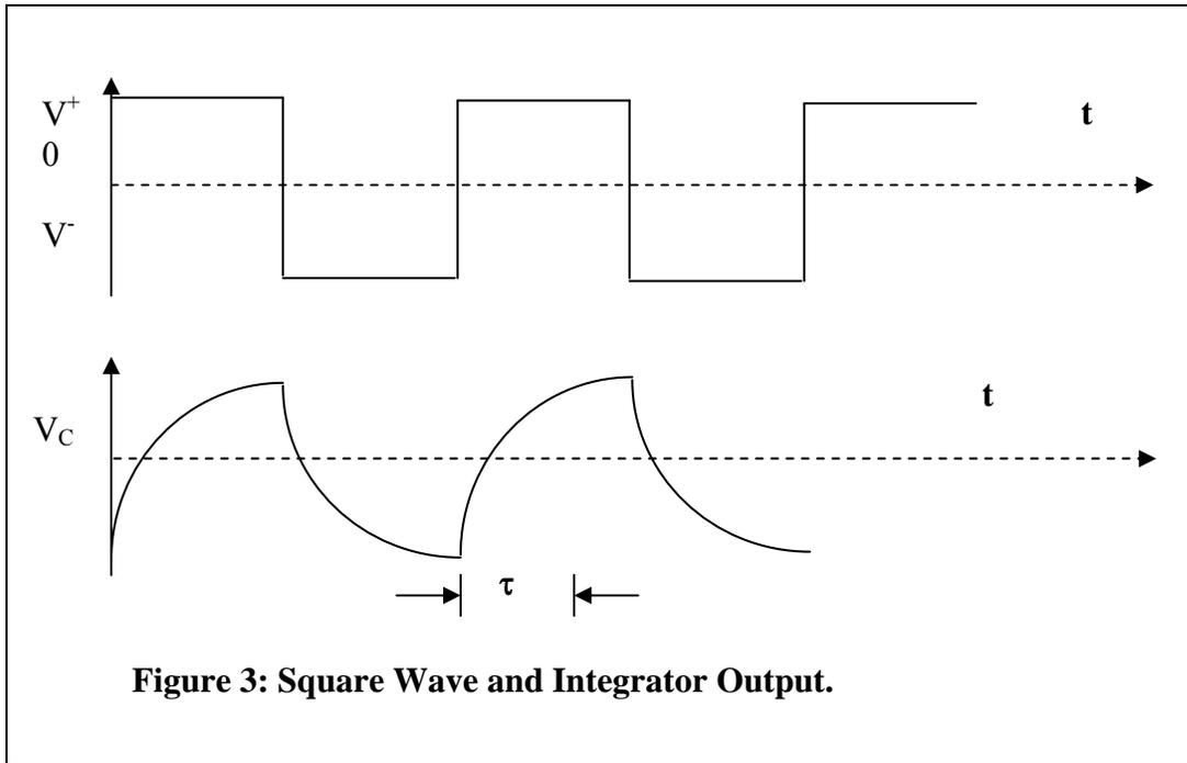
Use the vertical cursors of your DPO to measure the time required to rise to a value of  $(V_+ - V_-)(1 - e^{-1})$ . Accuracy in this measurement is improved if the pattern nearly fills the screen. This rise time must be equal to  $\tau$ . Compare with the calculated value of  $\tau$ .
