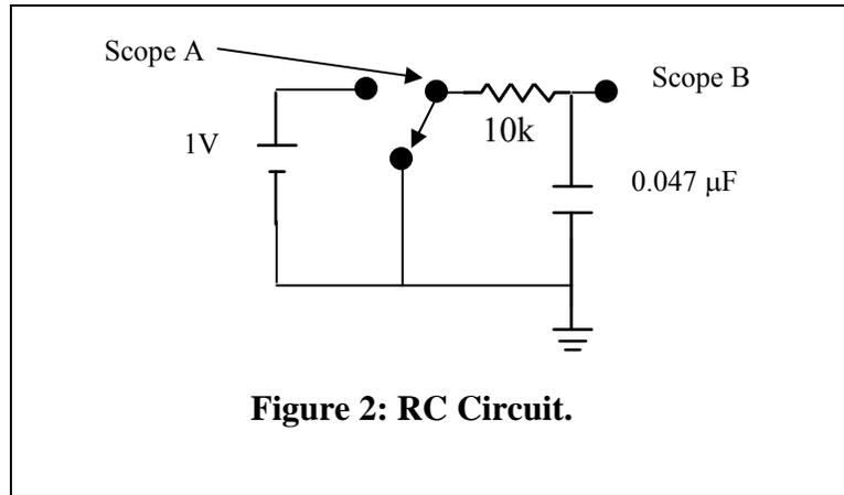
**Figure 2: RC Circuit.**
