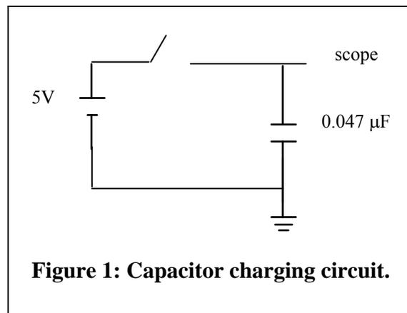
**Figure 1: Capacitor charging circuit.**
