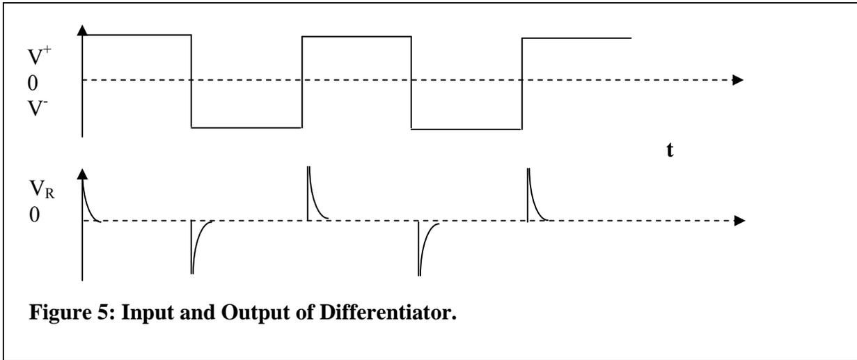
**Figure 5: Input and Output of Differentiator.**
