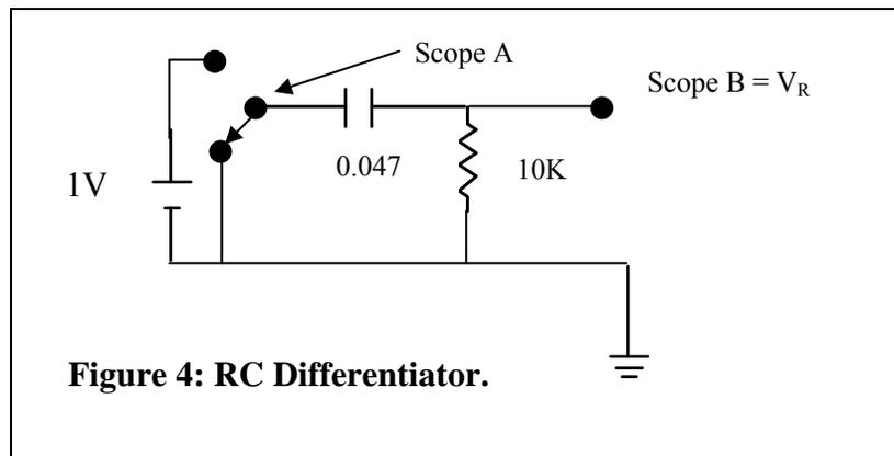
The output is the voltage across the resistor, which is the current, or  $dq/dt$  multiplied by the resistance  $R$ . Show that the solution for this voltage, consistent with no initial charge on the capacitor, is  $V_R = V_0 e^{-t/\tau}$ , where  $\tau = RC$ .
