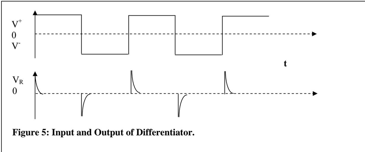
**Figure 5: Input and Output of Differentiator.**
