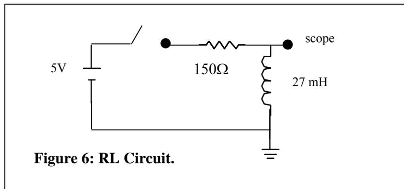
**Figure 6: RL Circuit.**
