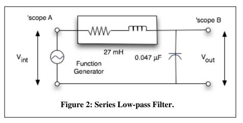
of the inductor plus any resistance contributed by the Function Generator. Normally the Function Generator has an output impedance of 50  $\Omega$ . Verify that this is the case by measuring the resistance of the function generator output with the generator turned on but the output voltage set to 0 V. Measure the resistance of the inductor, add the value contributed by the Function Generator and use this sum in your calculations below.
