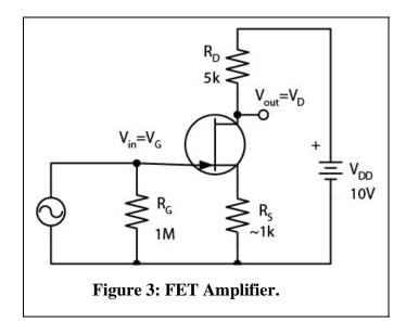
The circuit above is an AC amplifier. The output signal at the drain will be larger than the input signal on the gate.
