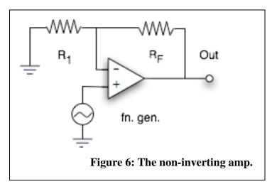
(a) \*Show mathematically that you expect the gain to be given by  $1+R_F/R_1$ . Measure the gain to verify this using resistor values in the range 3K to 200K. Paste a copy of an example DPO screen in your notebook.
