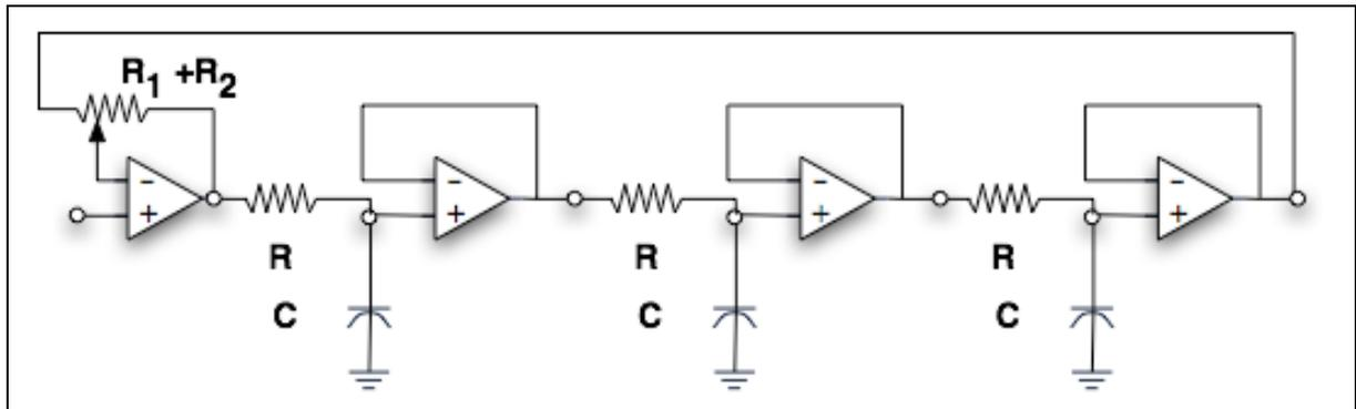
\*Show that the transfer function for the low pass resonant filter, shown in Figure 2, is given by:
