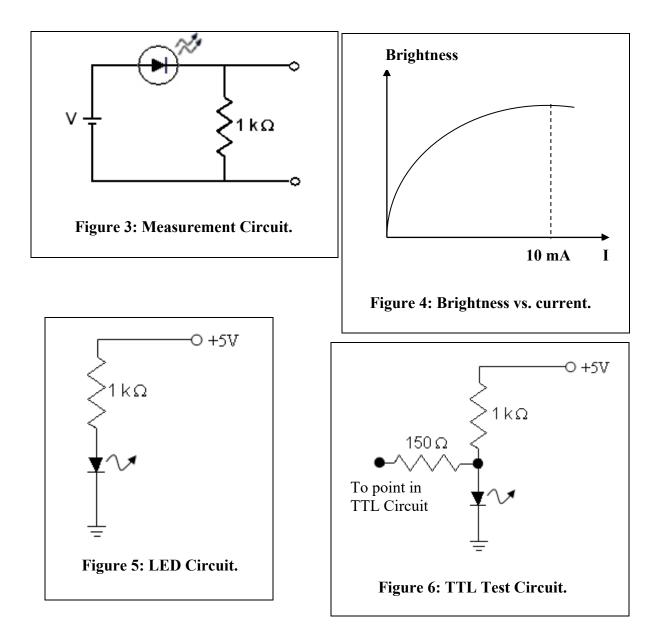
typical forward voltage drop for an LED within the red-green color range. Blue and white LEDs are characterized by higher voltage drops.
