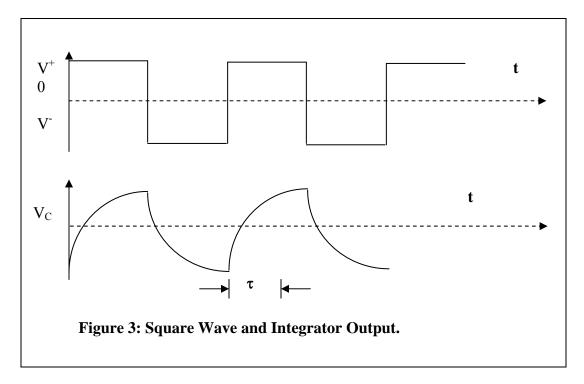
Use the vertical cursors of your DPO to measure the time required to rise to a value of  $(V_+ - V_-)(1-e^{-1})$ . Accuracy in this measurement is improved if the pattern nearly fills the screen. This rise time must be equal to  $\tau$ . Compare with the calculated value of  $\tau$ .
