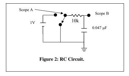
In lecture you learned that this circuit can be described by a differential equation for q(t), the charge on the capacitor as a function of time. It was shown that a solution for the voltage on the capacitor,  $V_C = q(t)/C$ , consistent with no initial charge on the capacitor, is:
