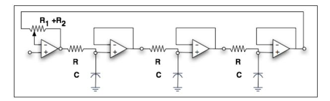
Figure 2: Low-pass Resonant Filter
