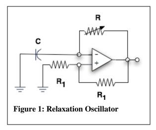
Build the relaxation oscillator shown in Figure 1 above. The output should be a square wave with a frequency about 1/(2RC). Resistor  $R_1$  can be any value between  $1k\Omega$  and  $1M\Omega$ . Resistor R is one side of a potentiometer. Examine the voltages at (+) and (-) inputs and at the output and follow the action of the switching. It is useful to display  $v_+$  and  $v_-$  simultaneously on the same scale to illustrate that the switching occurs at the crossover of  $v_+$  and  $v_-$ .
