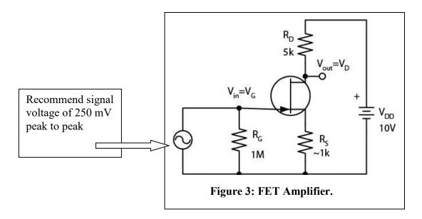
The circuit above is an AC amplifier. The output signal at the drain will be larger than the input signal on the gate.
