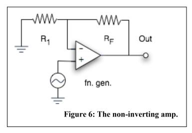
(a) \*Show mathematically that you expect the gain to be given by  $1+R_F/R_1$ . Measure the gain to verify this using resistor values in the range 3K to 200K. Paste a copy of an example DPO screen in your notebook. [4 p]
