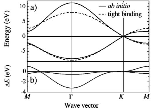
FIG. 2. *Ab initio* and nearest-neighbor tight-binding dispersions of graphene. (a) The converged *ab initio* calculation of the graphene  $\pi$  and  $\pi^*$  electronic bands is shown by the full lines. The dashed lines represent the tight-binding dispersion of Eq. (6) with  $s_0 = 0$  and  $\gamma_0 = -2.7$  eV. (b) Difference  $\Delta E$  between the *ab initio* and tight-binding band structures.
