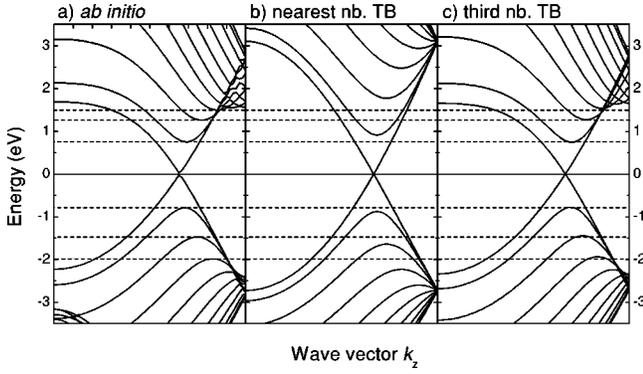
FIG. 4. Band structure of a (10,10) armchair nanotube. (a) *Ab initio* calculation. (b) Nearest-neighbor tight-binding calculation with  $\gamma_0 = -2.7$  eV. (c) Third-nearest-neighbor tight-binding calculation with parameters obtained from a fit to the optical energy range; see Table I. The dashed lines denote *ab initio* calculated energies of the singularities in the density of states.
