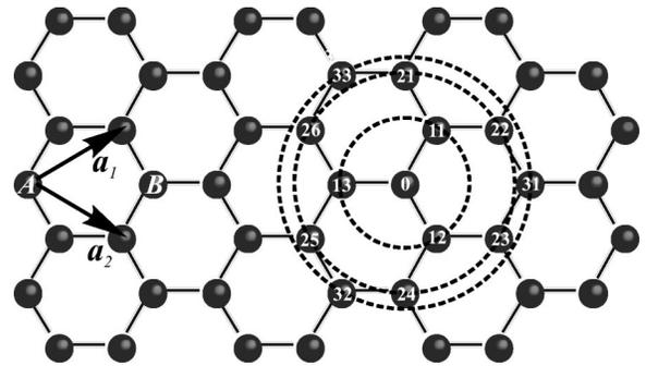
FIG. 1. Graphene hexagonal lattice.  $\mathbf{a}_1$  and  $\mathbf{a}_2$  are the unit-cell vectors of graphene with a lattice constant  $a = 2.461$  Å. The unit cell contains two carbon atoms  $A$  and  $B$  belonging to the two sublattices. An atom  $A_0$  has three nearest neighbors  $B_{1i}$ , six next-nearest neighbors  $A_{2i}$ , and three second-nearest neighbors  $B_{3i}$ .
