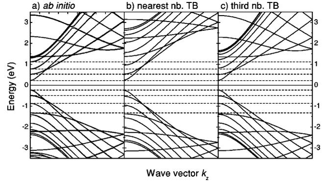
FIG. 5. Band structure of a (19,0) zigzag nanotube. (a) *Ab initio* calculation. (b) Nearest-neighbor tight-binding calculation with  $\gamma_0 = -2.7$  eV. (c) Third-nearest-neighbor tight-binding calculation with parameters obtained from a fit to the optical energy range; see Table I. The dashed lines denote *ab initio* calculated energies of the singularities in the density of states.
