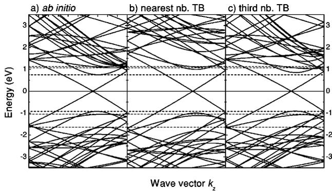
FIG. 6. Band structure of a (12,3) chiral nanotube. (a) *Ab initio* calculation. (b) Nearest-neighbor tight-binding calculation with  $\gamma_0 = -2.7$  eV. (c) Third-nearest-neighbor tight-binding calculation with parameters obtained from a fit to the optical energy range; see Table I. The dashed lines denote *ab initio* calculated energies of the singularities in the density of states.
