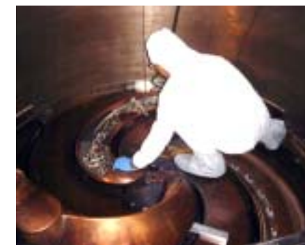
In this photo, the stripper foil mechanism has already been mounted inside the lower half of the "C" dee, and a cyclotron operator (in a "bunny suit" overall) is guiding the whole assembly into the K1200 cyclotron.
