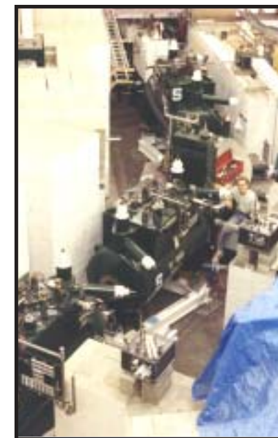
The first section of the A1900 beamline is shown. The exit beamline comes out of the K1200 vault at the top of the picture, and Cyclotron Operator Kevin Edwards is sitting on a part of the shielding wall that was under construction and still low at the time. Part of the first dipole is behind him (only the lower half is there), and the second triplet is next to him.
