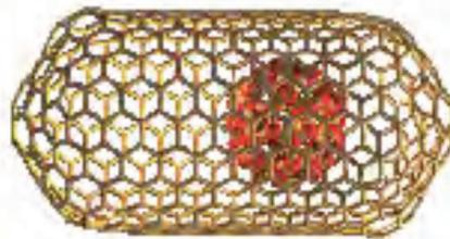
Fig. 2: A fullerene molecule inside a nanotube as a prototype non-volatile memory element capable of storing one bit information [U.S. Patent 6,473,351; *Phys. Rev. Lett.* **82**, 1470 (1999)].
