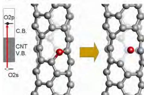
Fig. 3: Photo-induced de-oxidation of a defective carbon nanotube.
