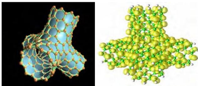
Fig. 1: Structural model (left) and spatial distribution of majority-spin electrons responsible for magnetism (right) in an all-carbon nanostructure [from *Phys. Rev. Lett.* **91**, 237204 (2003)].
