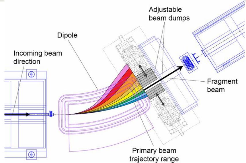
The fragmentation line beam dump model consists of two intersecting slabs.
