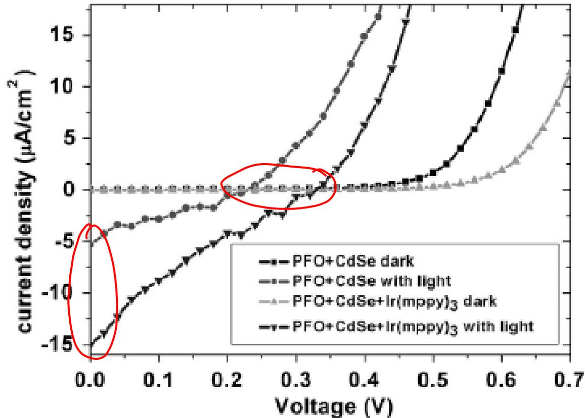
FIG. 2. Dark and photovoltaic responses of hybrid solar cells made from PFO/CdSe with and without Ir(mppy)<sub>3</sub>, showing 200% increase in short-circuit current and 50% increase in open-circuit voltage upon doping of Ir(mppy)<sub>3</sub>.
