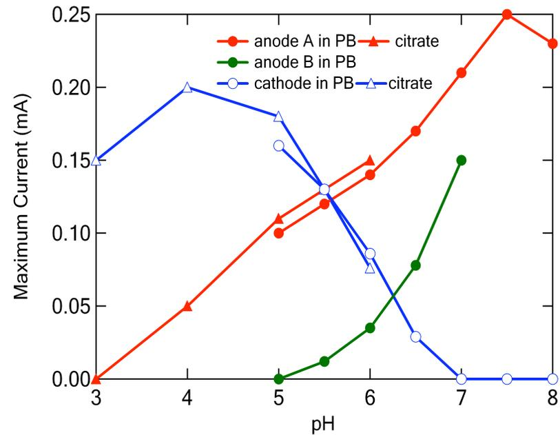
50 mM glucose, in 0.15 M buffer at 37.5 °C under air, flow rate 16 mL/min.
