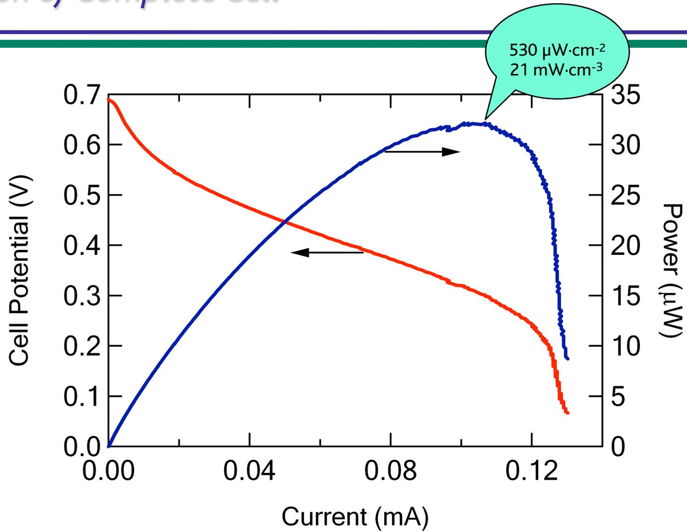
50 mM glucose, in 0.15 M, pH 5.5 citrate buffer at 37.5 °C under air, flow rate 16 mL/min. 6 mm × 1 mm × 0.25 mm electrode.
