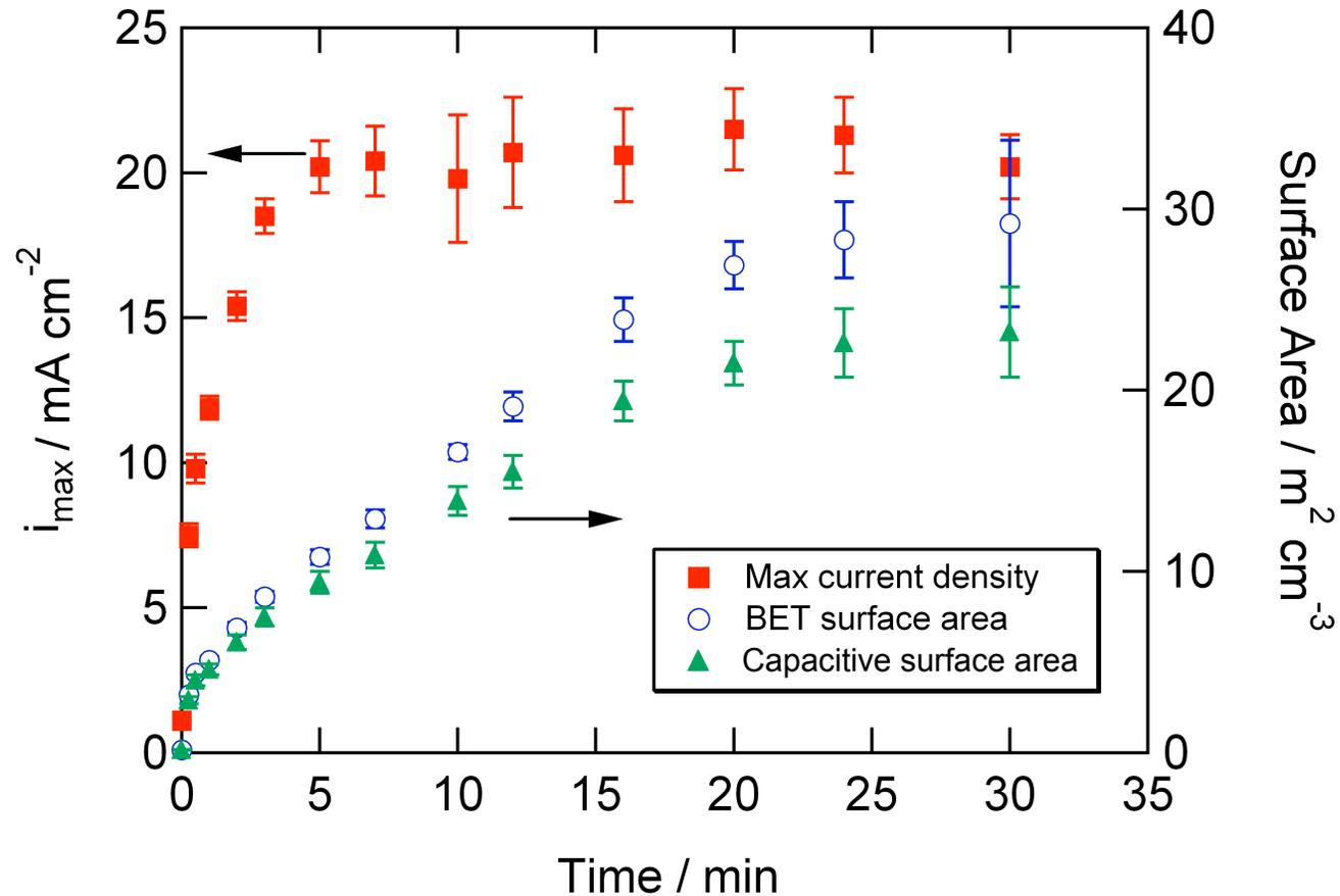
NT growth catalyzed with ohmic heating 90  $\mu\text{m}$  thick carbon paper substrate.
