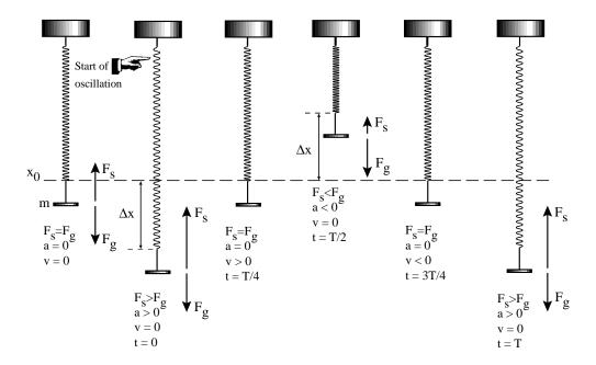
Figure 2: One cycle of an oscillation of the spring.
