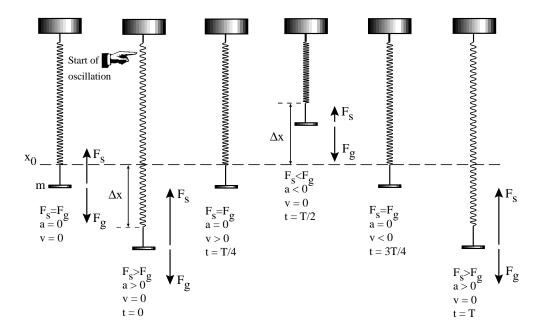
**Figure 1:** One cycle of an oscillation of the spring.
