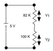
Figure 1: Resistors in Series.
