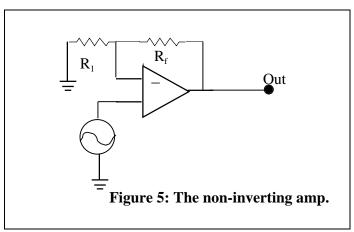
(a) Show mathematically that you expect the gain to be given by  $1 + R_f/R_1$ . Measure the gain to find out using resistor values in the range 3K to 200K.
