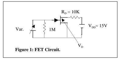
Now make the gate voltage more negative until the drain current is essentially zero. (Recognized because the drain voltage is almost as large as the supply  $V_{DD}$ .
