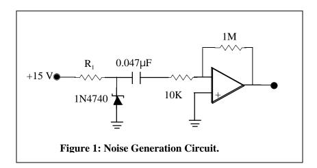
The strength and quality of the noise depends upon the diode and upon the current limiting resistor  $R_1$ . As a rule, high-voltage zeners work best. Because the power supply is 15 volts, a zener with breakdown voltage between 10 and 13 volts is recommended.
