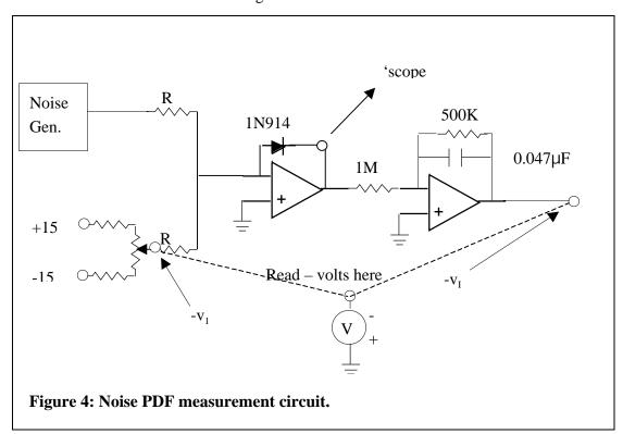
**Analysis**: When the sum of the noise voltage and the voltage called  $-v_1$  is negative the output of the comparator goes to a high state. When the sum is positive the output of the comparator goes to zero (or something close to zero). The leaky integrator integrates the
