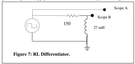
Calculate time constant = L/R. Remember to include the resistance intrinsic to the inductor in R. Measure the time constant on the 'scope.
