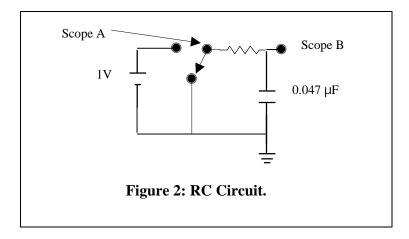
Write the differential equation for the voltage across the capacitor, as a function of time since the closing of the switch. The equation is effectively an equation for q(t), the charge on the capacitor.
