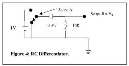
The output is the voltage across the resistor, which is essentially the current, or dq/dt. From your solution to the differential equation for the RC circuit show that a solution, consistent with no initial charge on the capacitor, is  $V_R = e^{-t/r}$ , where = RC.
