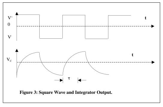
Use the 'scope to measure the time required to rise to a value of  $(V_+ - V_-)(1-e^{-1})$ .
