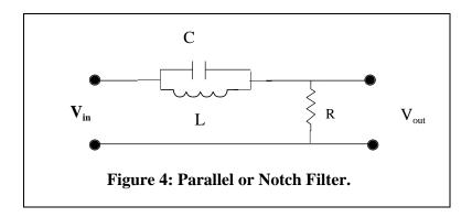
\* Explain why this is a notch filter. What is the frequency of the notch? Use L=27 mH, C=0.047  $\mu F$  and R=150 . Measure the depth of the notch by comparing the response at the bottom of the notch with the response at low or high frequency. Why doesn't the response go to zero at the bottom of the notch?
