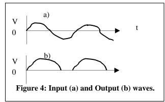
The basic half-wave rectifier with resistive load looks like the circuit above. The Input and Output waveforms are shown on the right.
