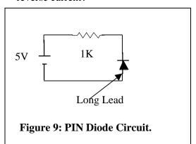
Reverse the diode to attempt to find the effect of light on the diode current in the forward-biased condition.
