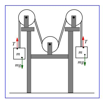
7. Equal masses are connected by a light string, and suspended by mass-less pulleys, as shown above. What is the tension in the string?
