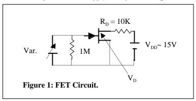
Now make the gate voltage more negative until the drain current is essentially zero. (Recognized because the drain voltage is almost as large as the supply  $V_{DD}$ .
