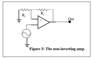
(a) Show mathematically that you expect the gain to be given by  $1+R_f/R_1$ . Measure the gain to find out using resistor values in the range 3K to 200K.
