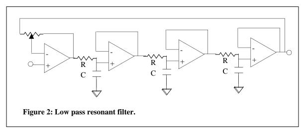
Show that the transfer function for the low pass resonant filter, shown in Figure 2, is given by:
