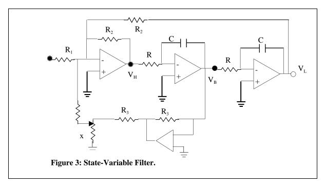
The state-variable filter has low-pass, band-pass, and high-pass outputs. The resonance frequency can be controlled with the time constant = RC, and the Q can be controlled independently.
