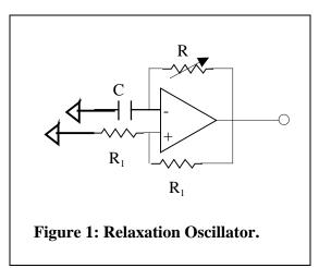
Build the relaxation oscillator shown in Figure 1 above. The output should be a square wave with a frequency about 1/(2RC). Resistor  $R_1$  can be any value between 1K and 1 M. Resistor R is one side of a potentiometer. Examine the voltages at (+) and (-) inputs and at the output and follow the action of the switching. It is useful to display  $v_+$  and  $v_-$  simultaneously on the same scale to illustrate that the switching occurs at the crossover of  $v_+$  and  $v_-$ .
