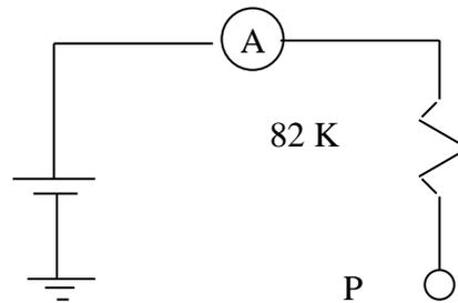
**Figure 2: Open Circuit.**
