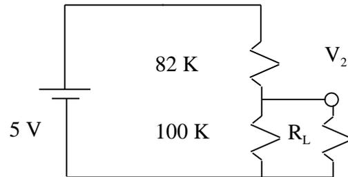
**Figure 3: Voltage Divider.**
