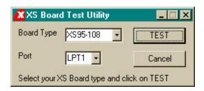
Your next step is to select the parallel port that your XS Board is connected to from the port pulldown list. GXSTEST starts with parallel port LPT1 as the default, but you can also select LPT2 or LPT3 depending upon the configuration of your PC.
