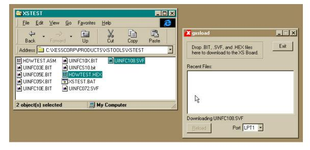
Once the downloading is finished, the file names are added to the Recent Files window and the Reload button is enabled. Now you can download these files to the XS Board just by clicking on the Reload button. This is a useful shortcut to have as you make changes to your design in Foundation and need to test the modifications.
