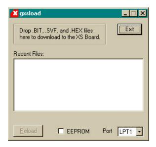
Your next step is to select the parallel port that your XS Board is connected to as shown below. GXSLOAD starts with parallel port LPT1 as the default, but you can also select LPT2 or LPT3 depending upon the configuration of your PC. If you are programming an XS40 Board with an Atmel serial EEPROM, you can also check the EEPROM box to enable the programming of the EEPROM. In most cases, however, you will leave the box unchecked so that the FPGA or CPLD on the XS Board will be programmed.
