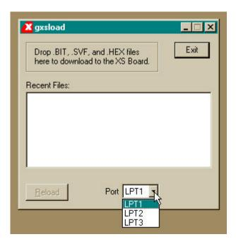
After setting the parallel port and EEPROM flag, you can download files to the XS Board simply by dragging them to the GXSLOAD window as shown below. Once you release the mouse left-button and drop the files, GXSLOAD will begin sending the files to the XS Board through the parallel port connection. If you drag & drop a non-downloadable file (one with a suffix other than .BIT, .SVF, or .HEX), GXSLOAD will ignore it.
