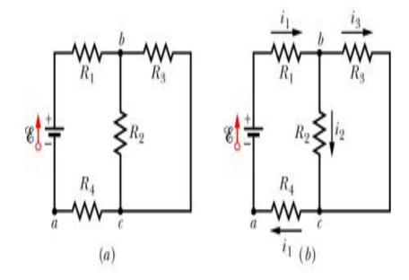
$$i_2 = \frac{V_2}{R_2}$$
