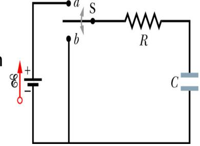
At t = 0 switch is open and capacitor is uncharged so q = 0
