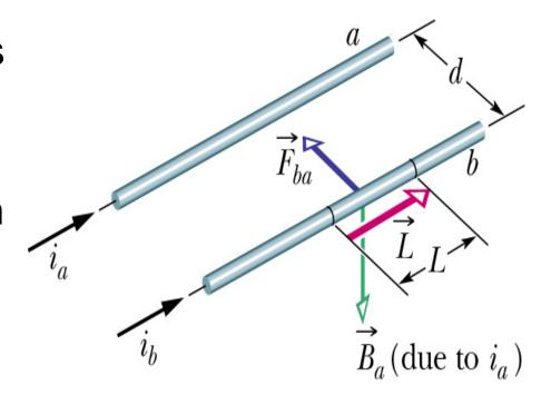
$$F_{ba} = i_b LB_a = \frac{\mu_0 L i_a i_b}{2\pi d}$$
