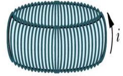
Use Ampere's law to calculate B field for a solenoid and a toroid
