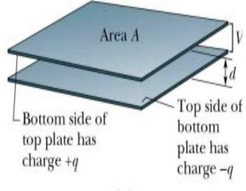
• C depends only on geometry of plates, not on their q or V
