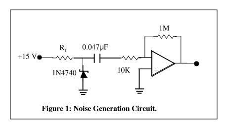
The strength and quality of the noise depends upon the diode and upon the current limiting resistor  $R_1$ . As a rule, high-voltage zeners work best. Because the power supply is 15 volts, a zener with breakdown voltage between 10 and 13 volts is recommended.
