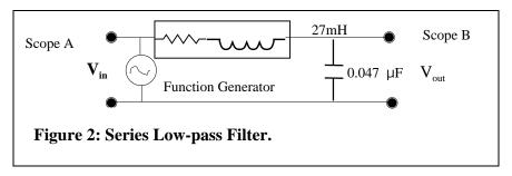
Notice that there is no discrete resistor. The resistor in this circuit is only the resistance of the inductor. Use an ohmmeter to measure the resistance of the inductor and use this value in your calculations below.
