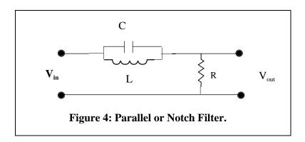
\* Explain why this is a notch filter. What is the frequency of the notch? Use L=27 mH, C=0.047  $\mu F$  and R=150 . Measure the depth of the notch by comparing the response at the bottom of the notch with the response at low or high frequency. Why doesn't the response go to zero at the bottom of the notch?
