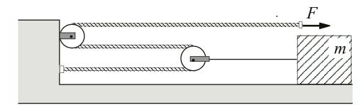
A massless rope runs through a pair of massless pulleys with a wire from one pulley to a mass, m, as shown in the figure above. A stationary person applies a force,  $\mathbf{F} = +F$ , to the end of the rope but due to frictional forces acting on the mass it does not move, i.e., the forces acting on the mass are balanced.
