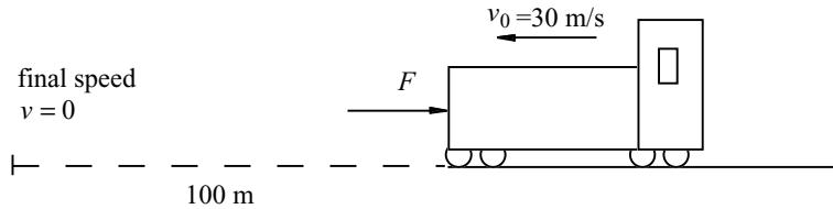
A train weighing  $10^6 \text{ N}$ , moving with a speed of  $30 \text{ m/s}$ , is slowed to  $v = 0$ , in a distance of  $100 \text{ m}$ , by a constant applied force,  $F$ .
