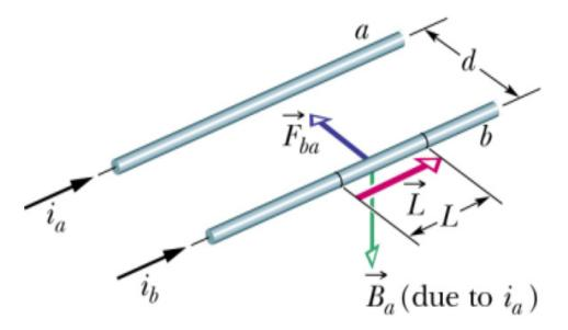
Applying right-hand rule, direction of F<sub>ba</sub> is towards wire a
