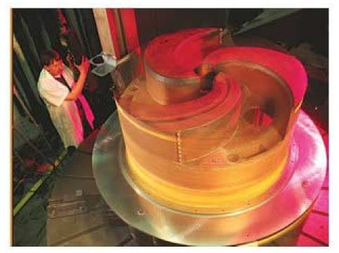
Machining the surface of the K500 cyclotron radiofrequency (RF) liner on a 10-foot-diameter vertical lathe. The RF liner is a thin copper shell that surrounds the magnets in the cyclotron and carries away excess power supplied by the radio frequency. Both cyclotrons currently operating at the NSCL have been designed and built in the laboratory.
