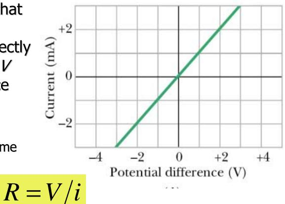
• A conducting device obeys Ohm's law when *R* is independent of size and direction of *V*
