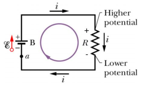
Could move around circuit counterclockwise
