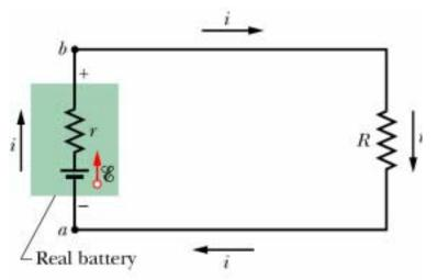
$$V_b - V_a = \mathsf{E} \frac{R}{R+r} = (12V) \frac{10\Omega}{10\Omega + 2\Omega} = 10V$$
