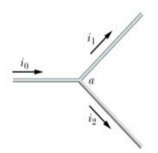
Current arrow drawn in the direction (+) charge carriers would move (actually it is the electrons that move).
