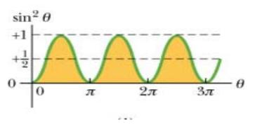
For alternating current circuits define rootmean-square or rms values for *i*, *V* and emf
