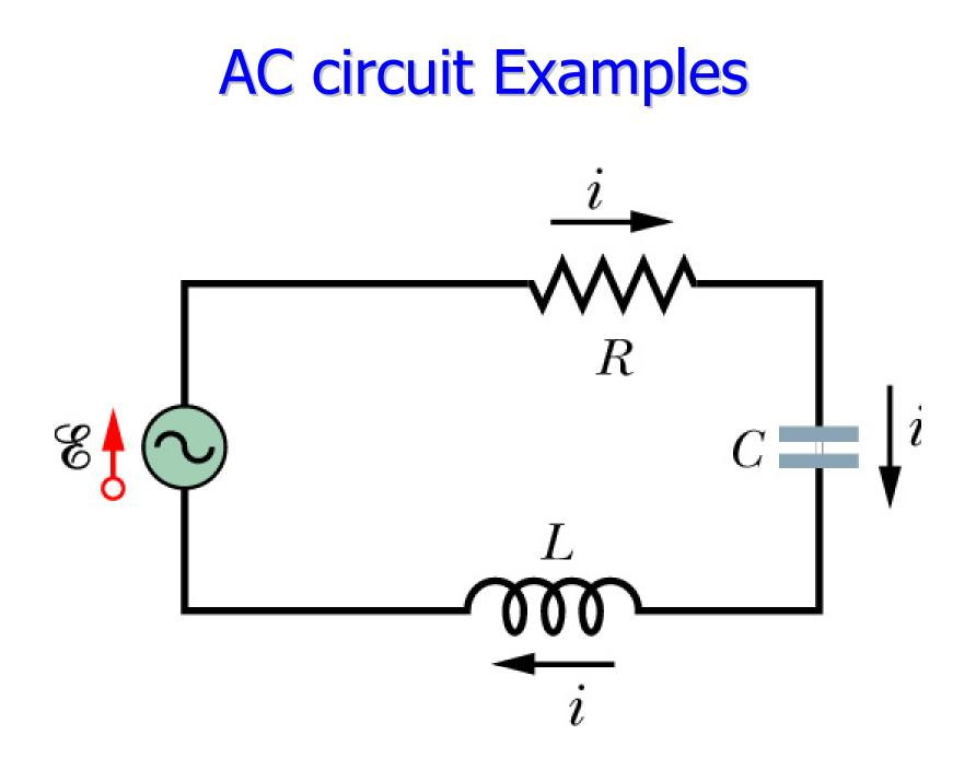
• Instantaneous rate which energy is dissipated (power) in a resistor is  $P = i^2 R$
