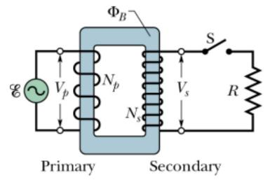
The current *I<sub>P</sub>* appears in primary circuit due to *R* in secondary circuit.
