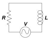
10. [3pt] What is the r.m.s. current (in amps) in the circuit above? DATA:  $L = 2.31 \times 10^{-1} H$ ,  $R = 55 \Omega$ ,  $V_{rms} = 110$ V, The frequency of the source is 60 Hz.
