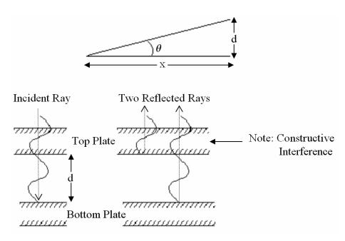
Because the beam reflected from the bottom of the film traverses the film twice, we see that the  $n^{th}$  bright fringe appears if
