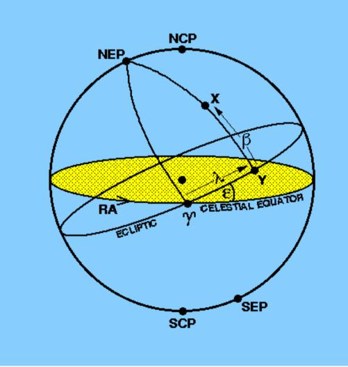
$\frac{Ecliptic \ Longitude}{A} (\lambda) - Measured \ along \ ecliptic from first point of Aries$
