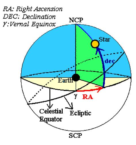
**<u>Right Ascension</u>** (RA) - angle measured in hours from the first point of Aries (24 hours = 360 degrees)
