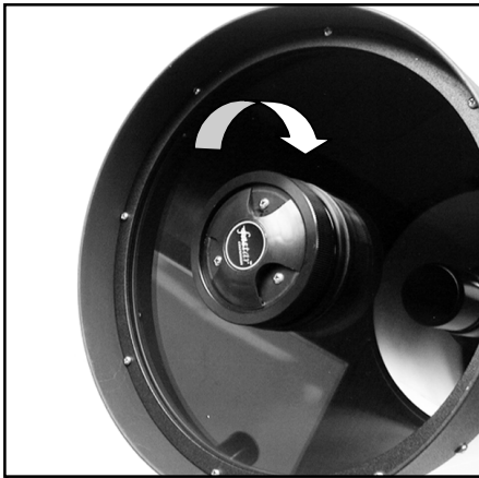
Figure 9-1 Rotate the collimation screw cover to access the three collimation screw.
