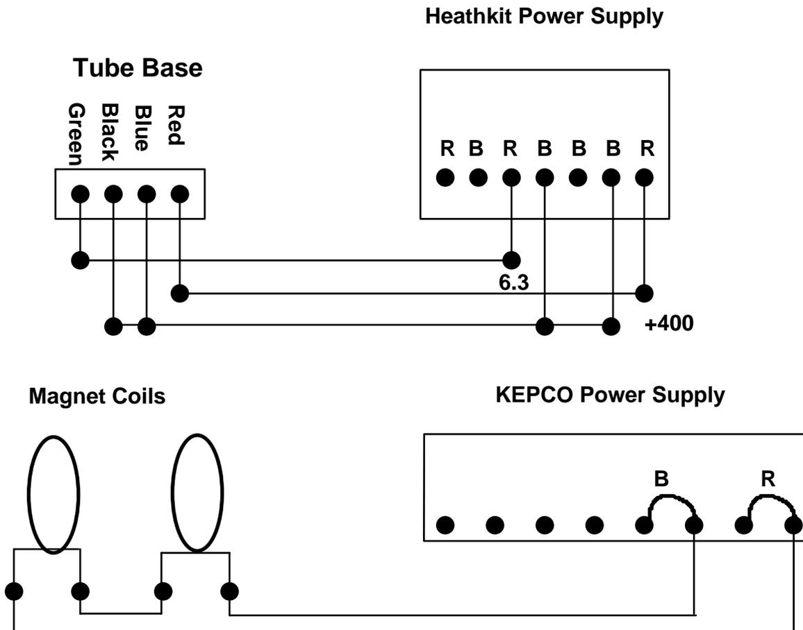
Note: The coils are connected "in series", but the correct "sense" will be determined by how the beam deflects
