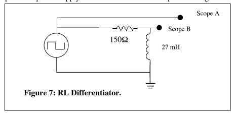
Calculate time constant  $\tau = L/R$ . Remember to include the resistance intrinsic to the inductor in R. Measure the time constant on the 'scope.
