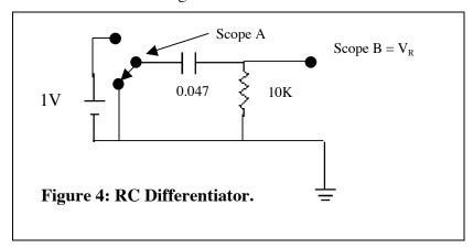
The output is the voltage across the resistor, which is the current, or dq/dt multiplied by the resistance R. If you have time, show that the solution for this voltage, consistent with no initial charge on the capacitor, is  $V_R = e^{-t/\tau}$ , where  $\tau = RC$ .
