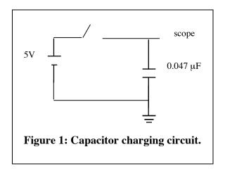
Next, replace the  $0.047~\mu F$  capacitor by a  $1000\mu F$  electrolytic capacitor [Pay attention to the capacitor polarity!] and watch the voltage across it after you disconnect the power supply. While you are waiting for something to happen, calculate the expected decay time. Come to a decision about whether you want to wait for something to happen. Act according to that decision.
