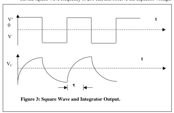
Use the 'scope to measure the time required to rise to a value of  $(V_+ - V_-)(1-e^{-1})$ . Accuracy in this measurement is improved if the pattern nearly fills the screen. This rise time must be equal to  $\tau$ . Compare with the calculated value of  $\tau$ .
