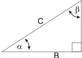
$$\begin{aligned}\sin \alpha &= \frac{A}{C}, \quad \cos \alpha = \frac{B}{C} \\ \tan \alpha &= \frac{A}{B}\end{aligned}$$
