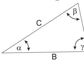
$$\begin{aligned}\frac{\sin \alpha}{A} &= \frac{\sin \beta}{B} = \frac{\sin \gamma}{C} \\ A^2 + B^2 - 2AB \cos \gamma &= C^2\end{aligned}$$
