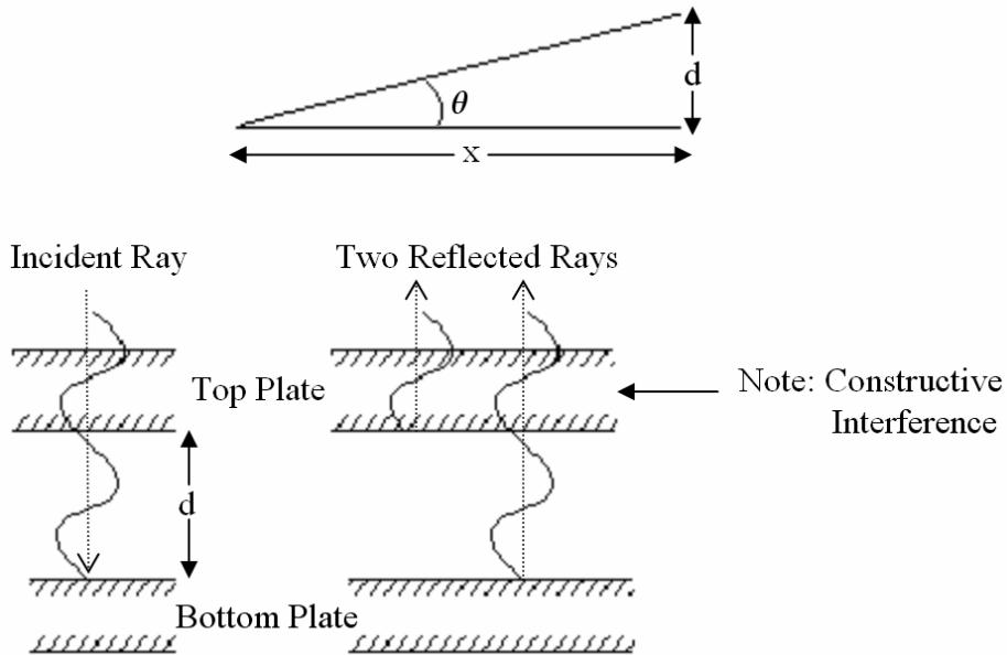
Because the beam reflected from the bottom of the film traverses the film twice, we see that the  $n^{\text{th}}$  bright fringe appears if
