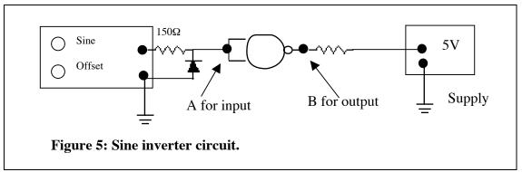
You should observe the output go low when the input sine goes above the switching voltage. You should observe the output go high when the input sine goes below the switching voltage.
