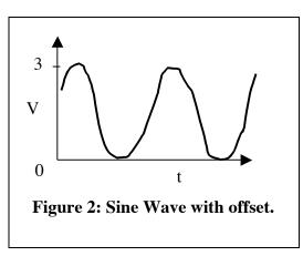
**Experiment**: Vary the level of the sine signal and the offset so that you see an output like Fig. 3. Then set the level and the offset so that the output resembles Fig. 2.
