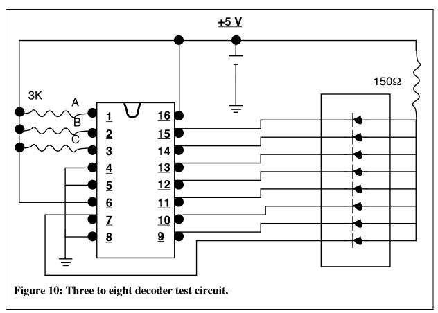
Experiment: Build the decoder shown in the figure below and verify its operation.
