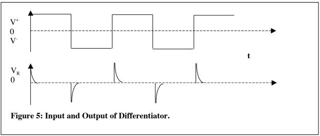
Now build the differentiator circuit, replacing the battery and switch by a square wave generator. Set the square wave frequency to 200 Hz, and observe the resistor voltage.
