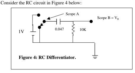
The output is the voltage across the resistor, which is the current, or dq/dt multiplied by the resistance R. If you have time, show that the solution for this voltage, consistent with no initial charge on the capacitor, is  $V_R = e^{-t/\tau}$ , where  $\tau = RC$ .
