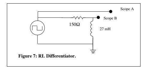
Calculate time constant  $\tau = L/R$ . Remember to include the resistance intrinsic to the inductor in R. Measure the time constant on the 'scope.
