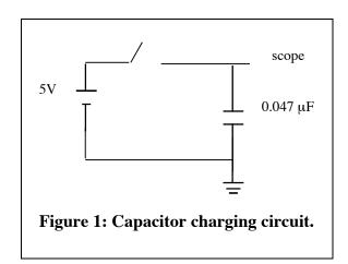
Next, replace the 0.047  $\mu$ F capacitor by a 1000 $\mu$ F electrolytic capacitor [Pay attention to the capacitor polarity!] and watch the voltage across it after you disconnect the power supply. While you are waiting for something to happen, calculate the expected decay time. Come to a decision about whether you want to wait for something to happen. Act according to that decision.
