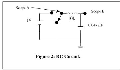
In lecture you will learn that this circuit can be described by a differential equation for q(t), the charge on the capacitor as a function of time. If you have time, you may wish to write down the equation and show that a solution for the voltage on the capacitor,  $V_c = q(t)/C$ , consistent with no initial charge on the capacitor, is:
